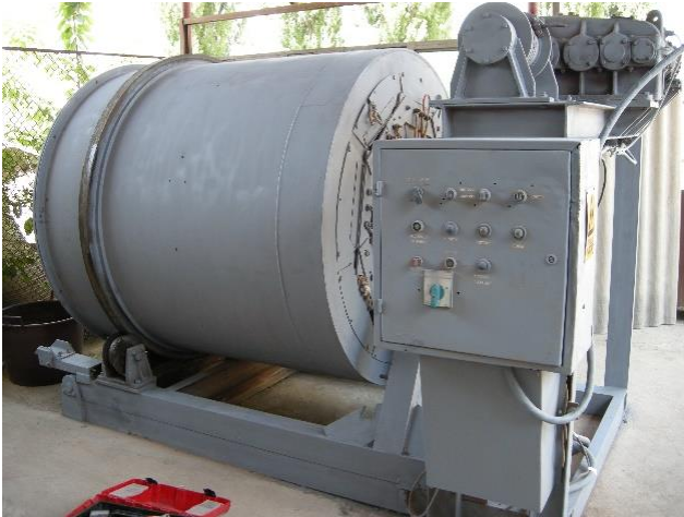
Figure 17. The experimental installation - rotary tubular furnace (Socalici A, 2016; Constantin N, et al., 2021; Project no. 233, 2008; Project no. 232, 2008)
