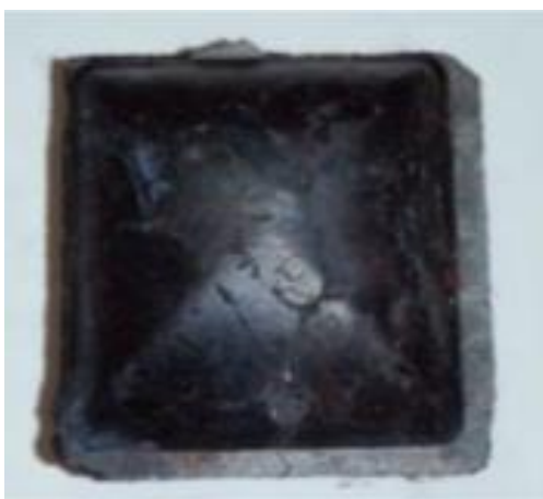
Figure 11. Lighter made of iron sponge manufactured by the FASTMET process (Tsutsumi H, et al., 2010).
