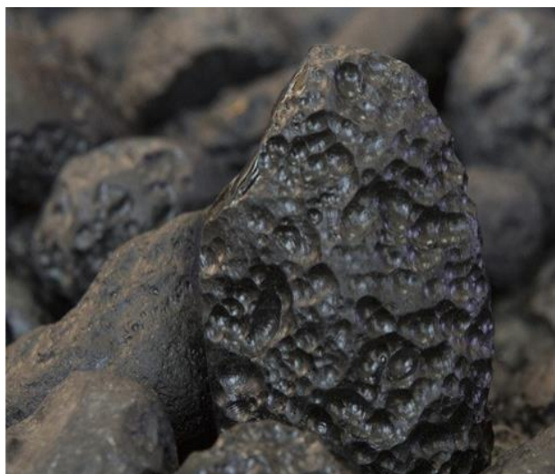
Figure 2. Iron sponge or direct reduced iron (FutureX Holding Limited, 2024)
